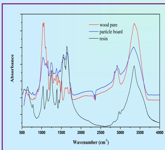
The FTIR absorbance spectra, obtained from small areas of the resin modified particle board present, except of the characteristic peaks of the resin, peaks attributed to the functional groups of the pure wood such as O-H (3600-3200 cm<sup>-1</sup>), C=O acetyl in xylans (1735cm<sup>-1</sup>), aromatic ring (1508, 1423, 1340-1315cm<sup>-1</sup>)
