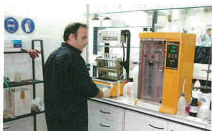
Using the Kjeldahl system for analysing the molar ratios of resins
