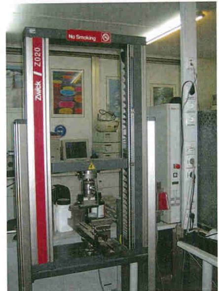
Left: Ultra Violet Visible Spectrophotometer testing. Above: Zwick equipment for testing a panel's mechanical strength
