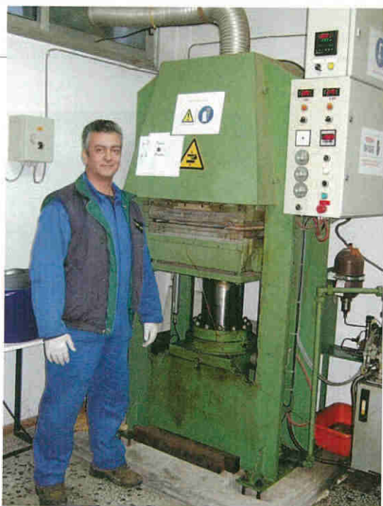
Left: The computerised 50x50cm press. Above: The particleboard blender, both at Chimar Hellas' pilot plant
