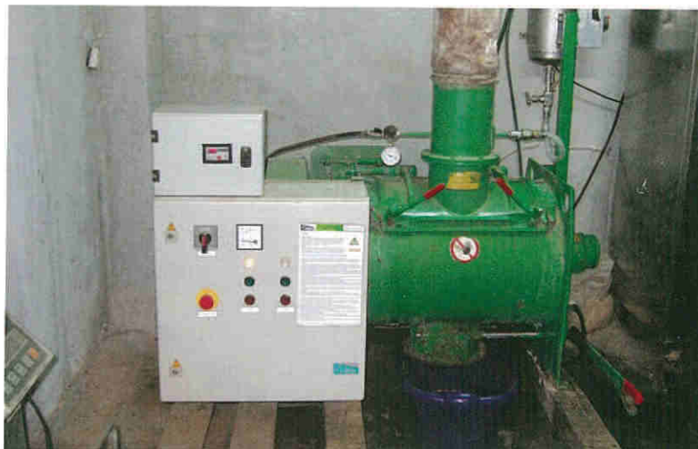
Left: The computerised 50x50cm press. Above: The particleboard blender, both at Chimar Hellas' pilot plant
