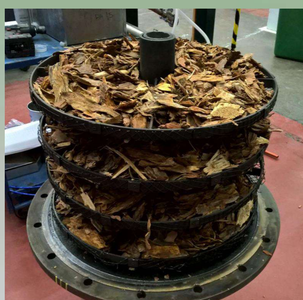
Figure 1. The sample holders that go inside the reactor filled with pine bark
