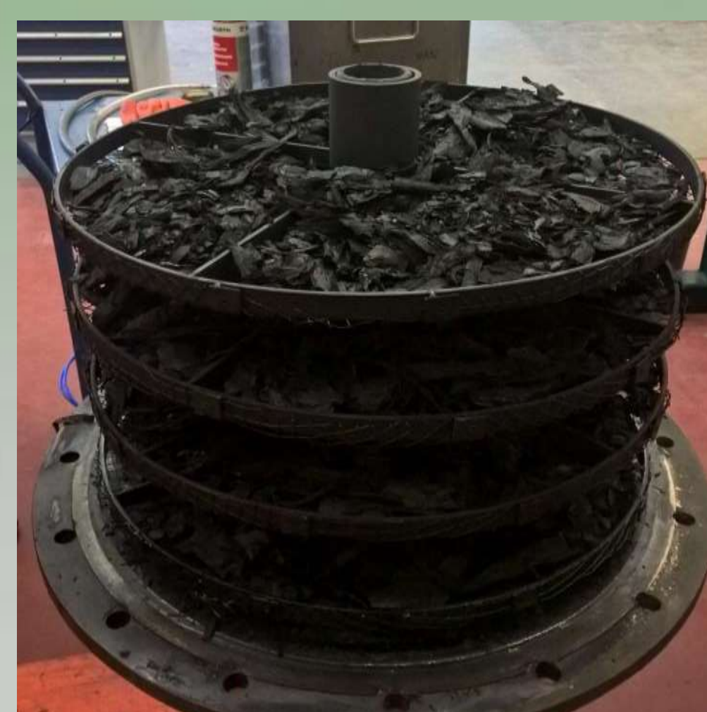
Figure 2. The sample holders after the test filled with pine bark biochar
