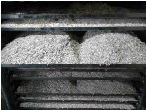
Drying of chips in the oven
