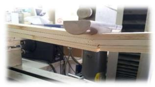
**Picture 2**: Testing of 3-lumber specimens, 100% wood failure
