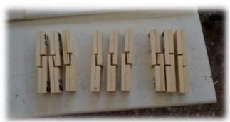
Picture 1: Laminated timber assembling
