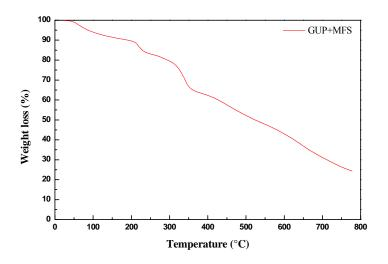
Figure 1: TGA curve of the flame retardant substance.
