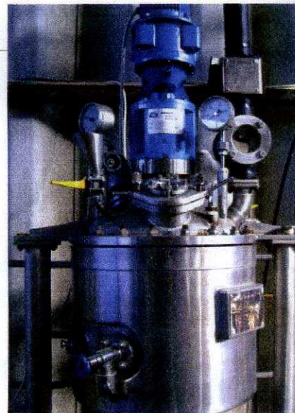
Pilot resin reactor, capacity 50 litres
