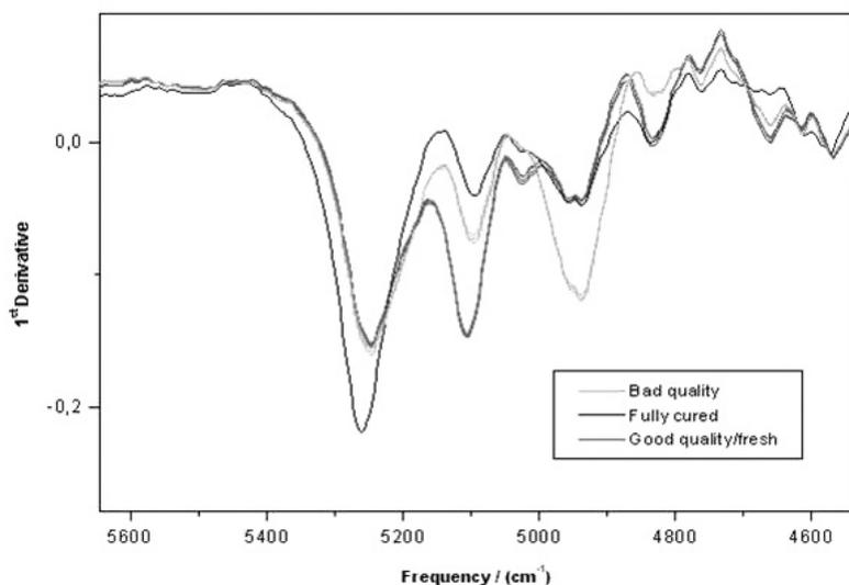
For the evaluation of laminating papers a quick and reliable conformity test has been developed based on NIR spectra acquired from paper samples in the diffuse reflectance mode. An empirical usability index has been built to detect the state of impregnated papers in a semi quantitative manner and report on its ability to be used [4-5].
