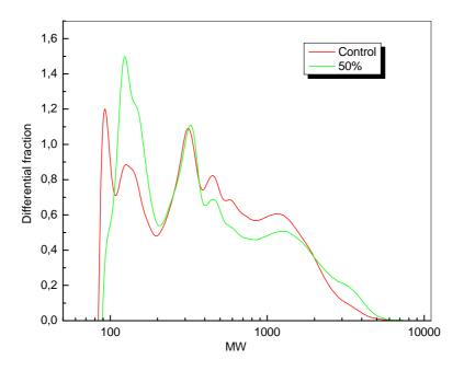
Graph 1: MWD of control and liquefiat modified PF resin
