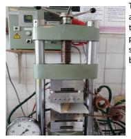
The bonding strength of this adhesive system has been tested by applying it to the preparation of small 3-ply specimens using 2.5x15cm birch strips.
